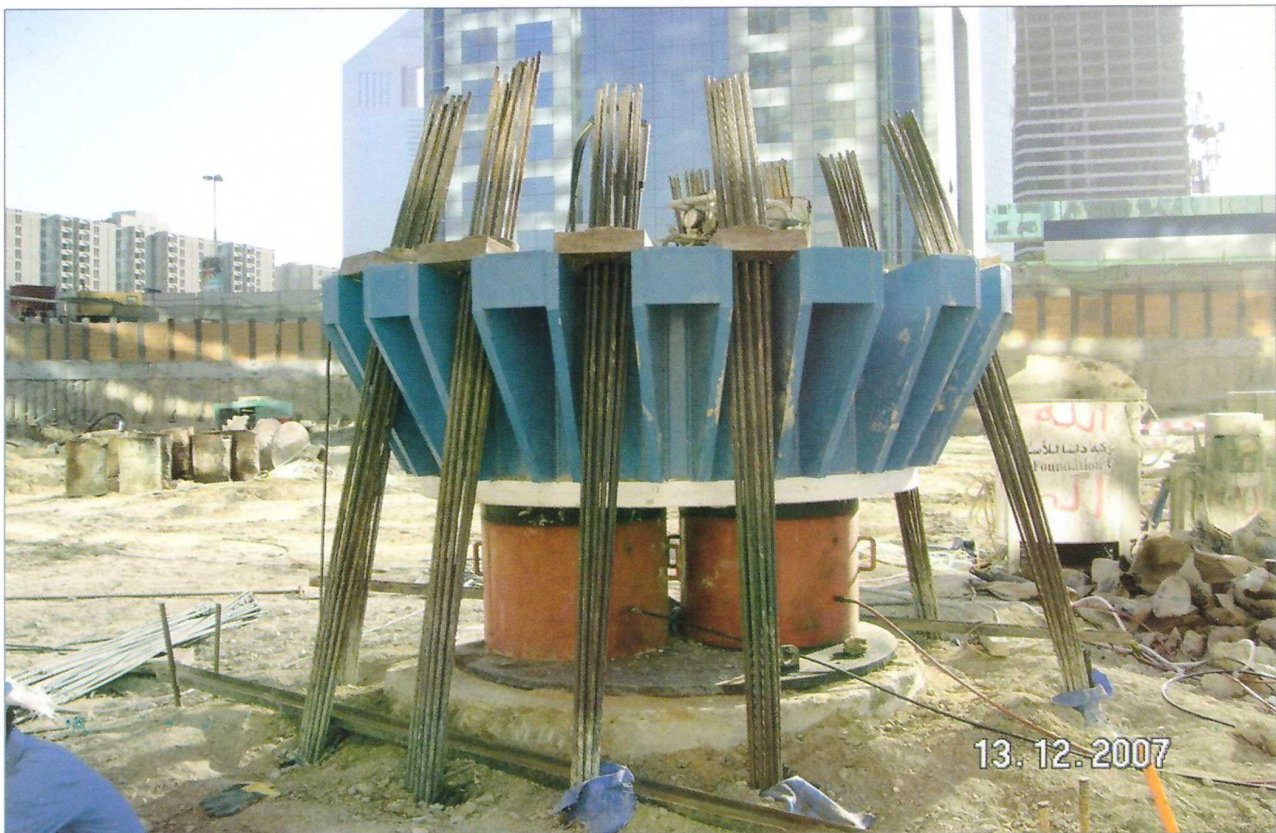
Static compression load test of 3270 Ton done at Conrad Hotel Project site at Shk. Zayed Road.
