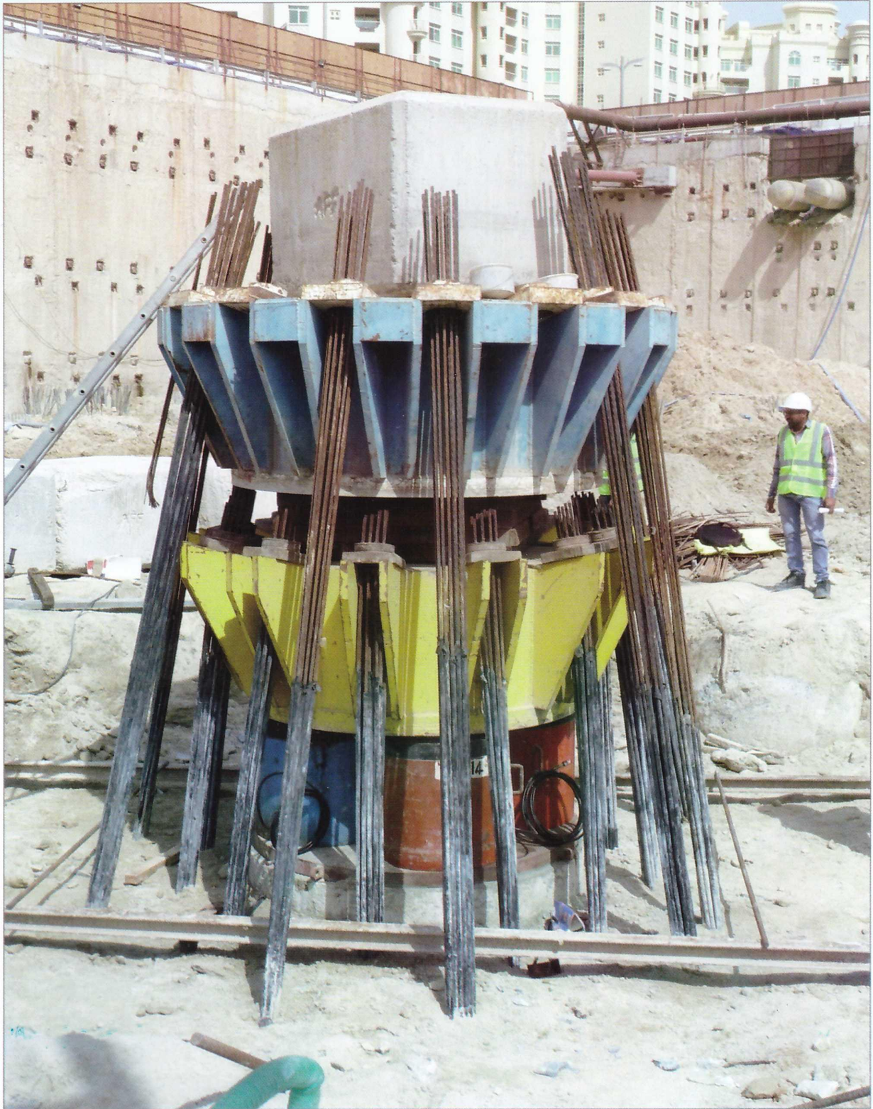
Static compression load test of 4350 Ton done at Nakheel Mall Project site in Palm Jumeirah.
