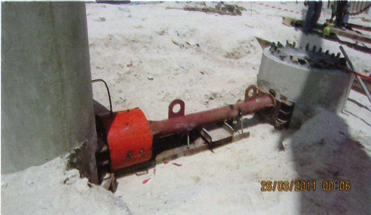
Horizontal lateral pile load test of 150 Ton done at Gulf Jyoti Foundation site at Jabel Ali.
